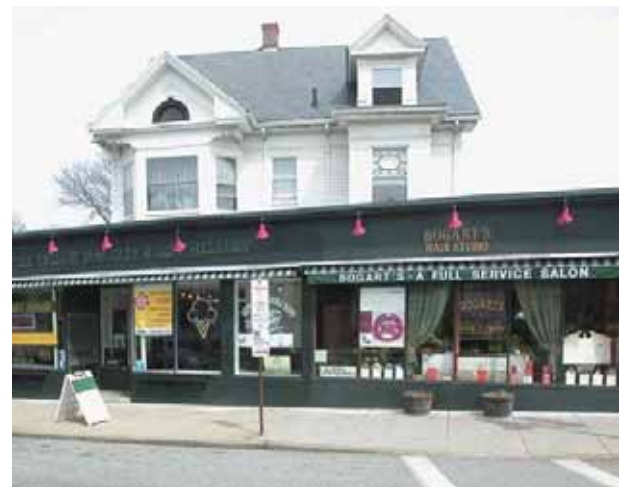
Because the retail addition here is set forward of the historic residence it can be treated as a separate building in color and architectural treatments.
